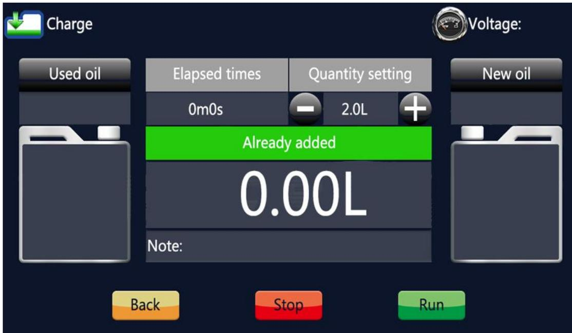
Set the required amount of replenishment on this interface before adding new oil, and press "Run".
